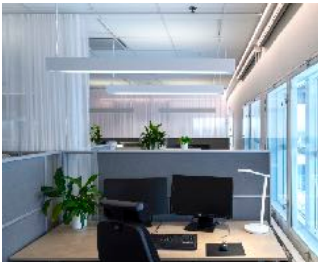
Schaeffler office refurbishment, Arlandastad, 2021. A line of light around the outer edge mimics the daylight colour shift
